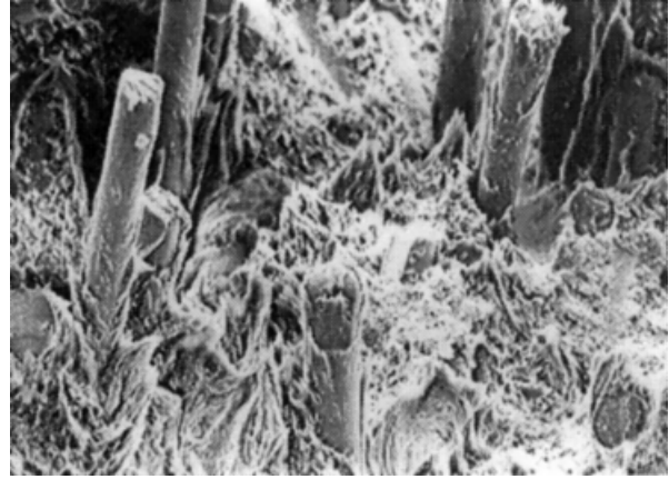
Figure 15 SEM micrograph of PBT/AX8900/SGF (60/10/30) compact tension specimen tested at 1 mm/min (700 x).
